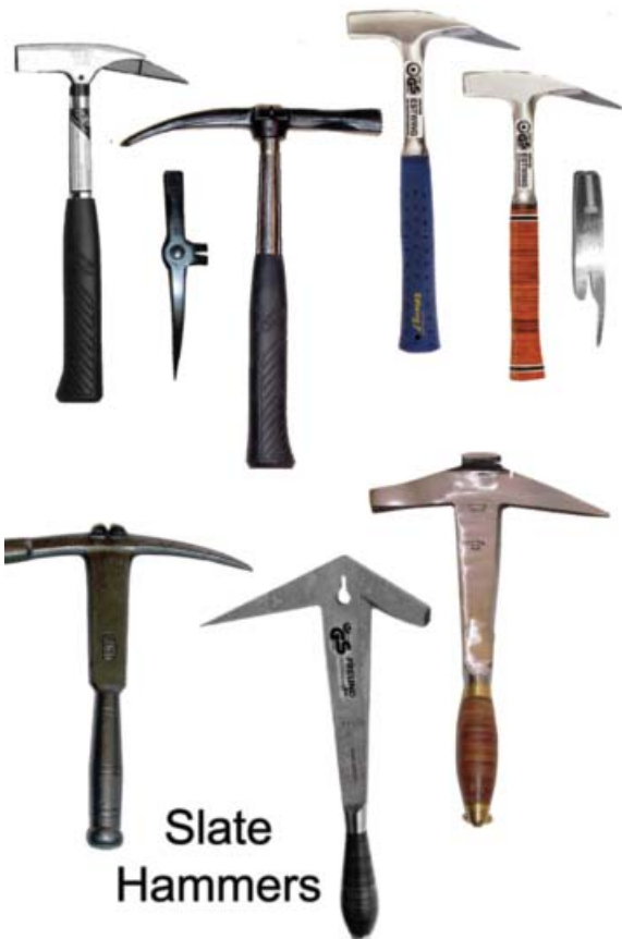
Figure 12: Slate hammers come in a variety of shapes and styles. They all have a pointed pick end that is used to punch nail holes in slates.
