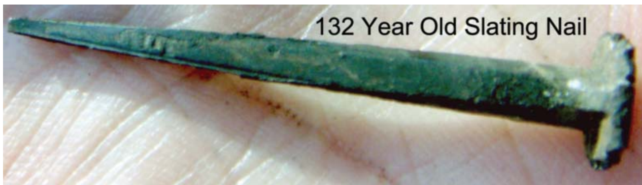
Figure 9: Just because the roof is old doesn't mean the nails have gone bad. This steel slating nail was pulled off a Buckingham slate roof on an 1879 church in Virginia in 2011. [Photo by Joseph Jenkins]
