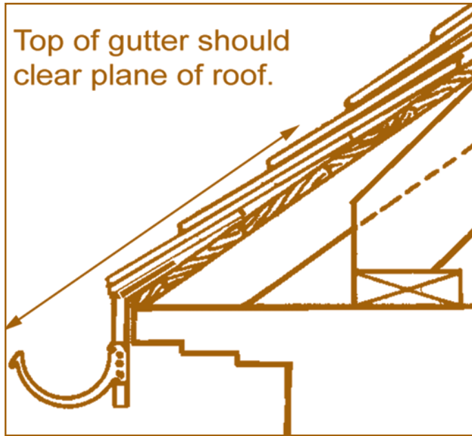
Figure 29 – Ideally, the outer edge of external rain gutters should be hung below the plane of the roof to prevent damage to the gutters from sliding ice and snow.
