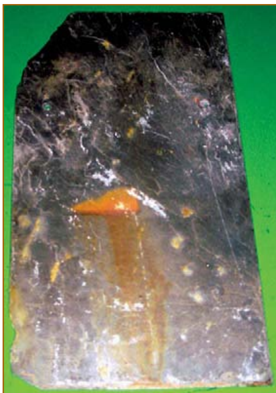
Figure 2 – This Spanish black slate leached rust stains down the new slate roof. This photo shows the slate after only one year on the roof.
