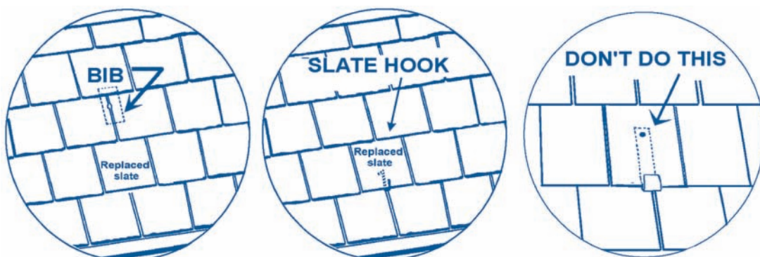
Figure 13: Standard methods for replacing slates in the field of the roof include the nail-in-slot and bib method (left) and the slate hood method (center). The exposed strap method (right) is to be avoided).
